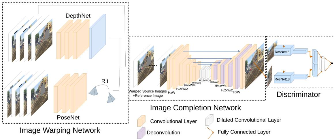
Fig. 1. **The proposed network architecture.** The proposed neural network architecture for multi-view assisted image completion. The proposed network consists of two components: Image Warping and Image Completion Network.
