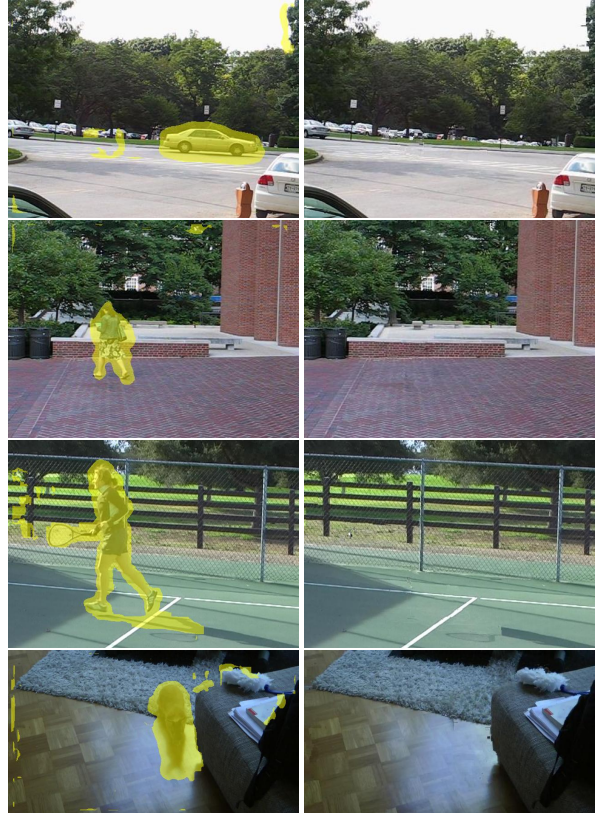
Figure 6. The figure shows the dynamic object detection and removal results obtained on the reference image of four multi-view image sets extracted from Freiburg Berkeley Motion Segmentation Dataset [5] using the proposed approach.
