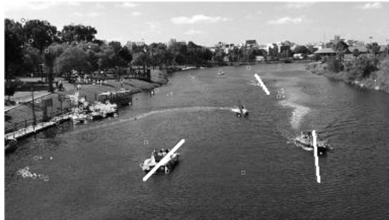
Fig. 4. Estimated curve through dynamic points which depict the sequence of captured images by camera 1.
